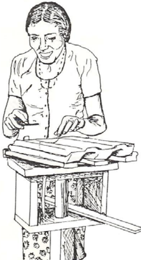
Figure 3: Trimming a tile on a rotating head stand. The stick on the stand is used for slapping the sides of the tile.
