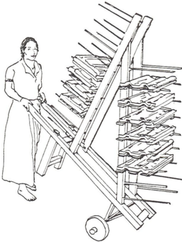
Figure 5: A cart for moving wet tiles.
